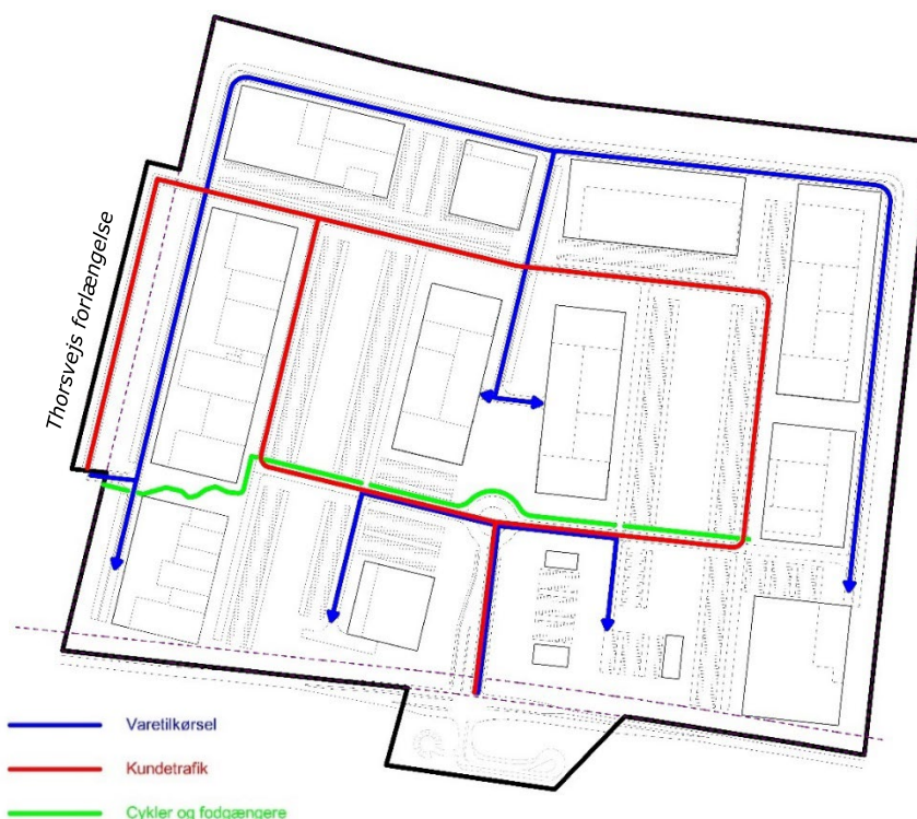
Figur 6-8 Vejbetjeningsprincipper for Grindsted Retail Park (Grindsted Retail Park Aps, Situationsplan, 2025).
